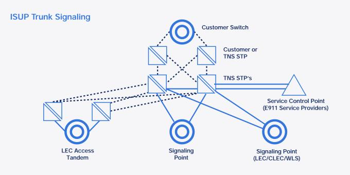
TNS ISUP - Service performs out-of-band call set-up and teardown and uses the same signaling path to facilitate inter-office CLASS services
